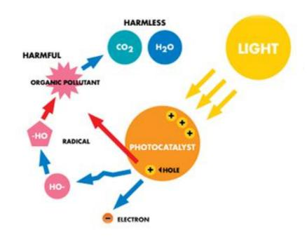
phenomenon whereby an active substance called a photocatalyst present on the surface of the filter, through the action of LED light placed on the sides, converts light energy into electrons, which from the reaction with the water present in the humidity of the air that passes through it causes a decomposition of the organic and inorganic pollutants present in the airflow, thus reducing the bacterial load.
